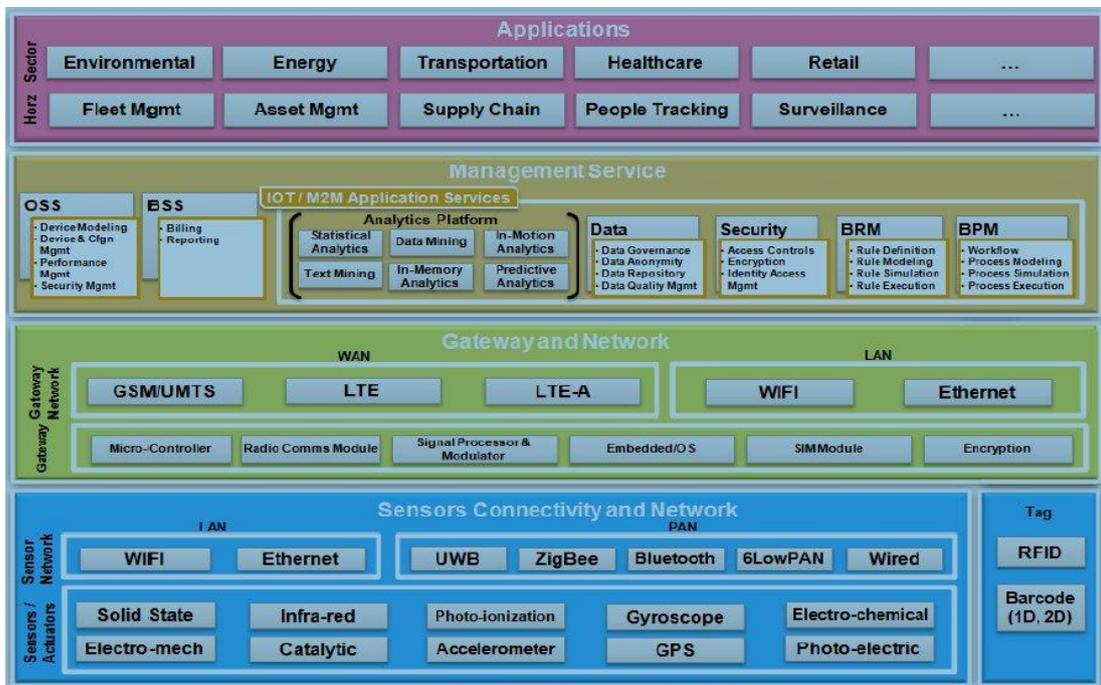
*Figure 1: IoT Architecture (Adapted from Ndubuaku & Okereafor, 2015)*
